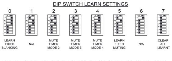
**Warning** The two hard-wired mute input connections to the light curtain must be disconnected when using the Learn mode.
