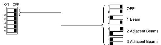
The floating blanking function is particularly useful for those applications where, for example, a work piece is moving up and down within the infrared field of the light curtain as part of the manufacturing process. This allows the operator to manipulate the work piece safely without shutting down the machine.
