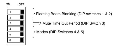
**Note**: If the parity or any of the DIP switches are changed while the light curtain is in operation the OSSDs (safety outputs) will turn OFF and remain OFF. All DIP switch setting must be done with the power to the light curtain disconnected. Refer to the Parity setting section.
