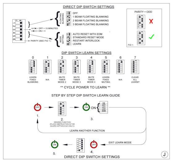
There are two modes of DIP switch setting for the T4 series:
