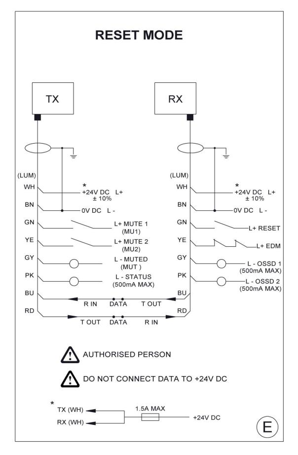
**Warning** Do not disconnect the cables from the Transmitter (TX) or Receiver (RX) head with the power still connected to the T4 (053B) series light curtain.
