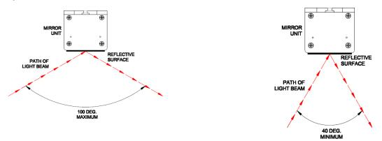
The angle of the infrared beams from the light curtain striking the reflective surface must be within defined limits as per the drawings above. See Fig. D in this guide.
