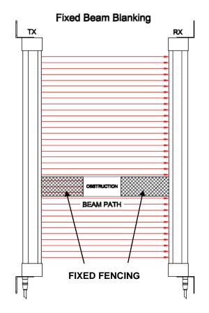
**Warning** If the fixed object located in the sensing region does not completely cover the light curtains sensing region additional guarding will be required.
